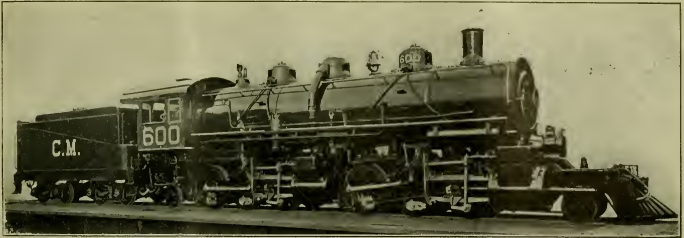
MALLET ARTICULATED COMPOUND LOCOMOTIVE FOR ROAD SERVICE—MEXICAN CENTRAL RAILWAY.
